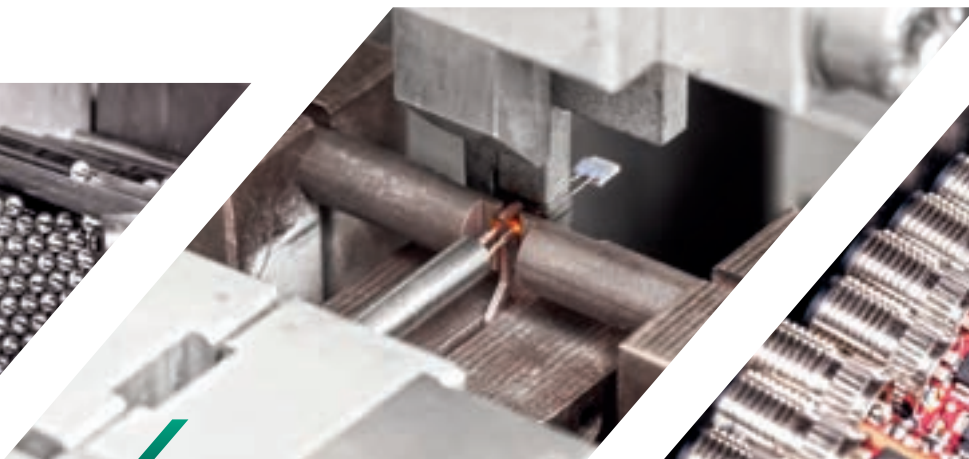
RTD automatic welding
